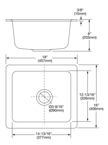
NOTES: \* DIMENSIONS SHOWN FOR LOCATION OF SUPPLIES AND "P" TRAP ARE SUGGESTED. FITTINGS NOT INCLUDED WITH FIXTURE AND MUST BE ORDERED SEPARATELY. SEALING COMPOUND SUPPLIED BY OTHERS.
